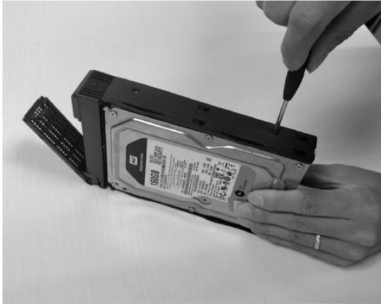
3.5" hard drive(4screws fixed on both sides)
