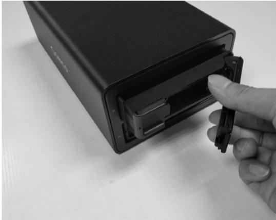
3. Install the 2.5 " /3.5" SATA HDD/SSD , secured with screws.
